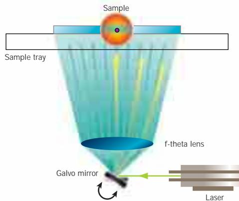
**Fig 9.** Moving-head scanning mechanism. The light beam from the laser is folded by a series of mirrors and ultimately reflected onto the sample. The sample is illuminated across its width as the scan head moves along the scan head rail (X-axis). The entire sample is illuminated by the scan head, laser, and mirrors tracking along the length of the sample (Y-axis).
