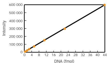
**Fig 5.** Fluorescence linearity. A 24-mer DNA oligonucleotide, 5' end-labelled with fluorescein (two-fold serial dilutions) was detected in a denaturing polyacrylamide gel sandwich using the Typhoon Imager with 532 nm excitation and 526 SP emission filter. The plot shows signal linearity over a range of 100 amol to 44 fmol.
