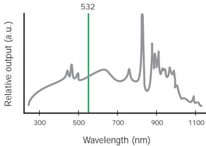
**Fig 7.** Spectral output of light from a xenon lamp and Nd:YAG laser. The “relative output” axis is scaled arbitrarily for the two light sources. The 532-nm line of the Nd:YAG laser is shown in green.
