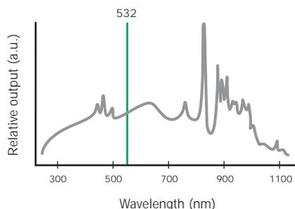
**Fig 71.** Spectral output of light from a xenon lamp and Nd:YAG laser. The “relative output” axis is scaled arbitrarily for the two light sources. The 532-nm line of the Nd:YAG laser is shown in green.
