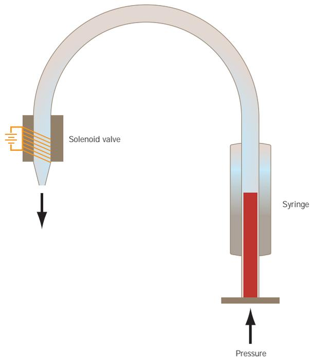
Fig 11. Diagram of a syringe-solenoid microarray printing system.
