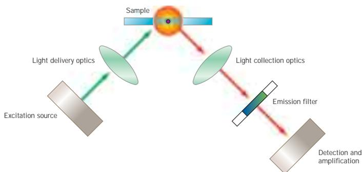
Fig 70. Components of a general fluorescence imaging system.
