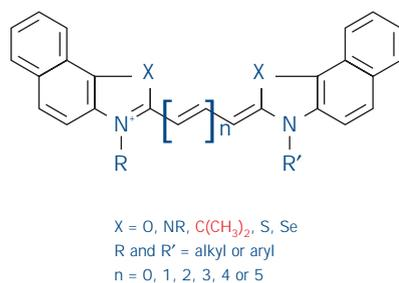
Fig 28. Core structure of the cyanine dyes.
