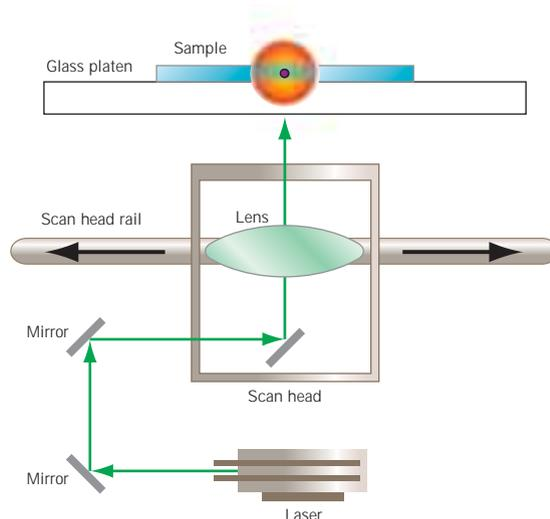
**Fig 73.** Moving-head scanning mechanism. The light beam from the laser is folded by a series of mirrors and ultimately reflected onto the sample. The sample is illuminated across its width as the scan head moves along the scan head rail (X-axis). The entire sample is illuminated by the scan head, laser, and mirrors tracking along the length of the sample (Y-axis).
