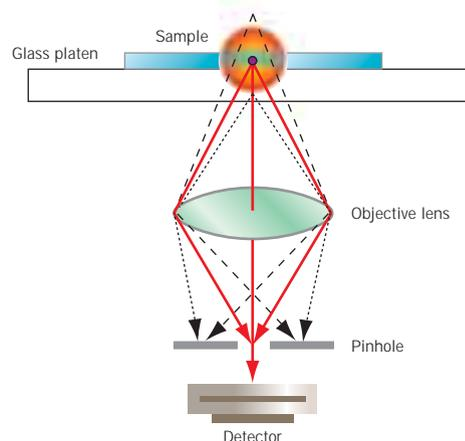
**Fig 74.** Illustration of confocal optics. Fluorescence from the sample is collected by an objective lens and directed toward a pinhole aperture. The pinhole allows the emitted light from a narrow focal plane (red solid lines) to pass to the detector, while blocking most of the out-of-focus light (black dashed lines).
