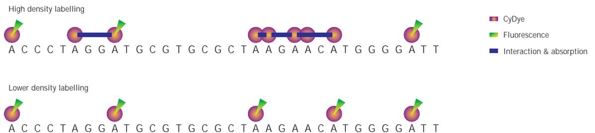
**Fig 26.** A schematic representation of the effect of quenching under varying labelling conditions. Fluorescent signal from the same nucleic acid fragment labelled with high and low densities is depicted. Green shows fluorescent emission, whereas purple denotes dissipation of energy between closely spaced fluors (pink circles).
