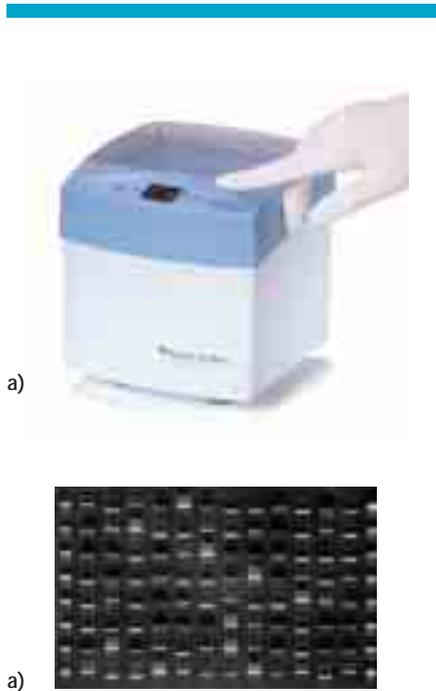
Fig 7. Separation of PCR\* fragments with Ready-to-Run Electrophoresis System.
